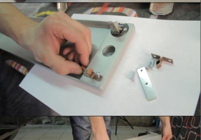
21. Mount opposite latch to license plate using M3 nut plate (14) and screws M3x12 (25).
