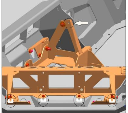
30. Using a 10mm drill bit drill a hole through the existing hole of the winch bracket from both left and right.
