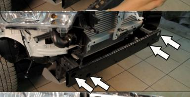
10. Remove 4xM10 bolts fixing crash beam to chassis. Set aside for re-use later on.
