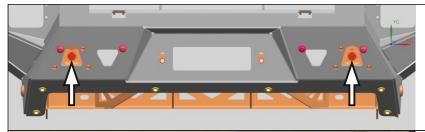
26. Give a few turns to M12x30 bolts (24) with M12x24 washers (38) which will assist with seating.
