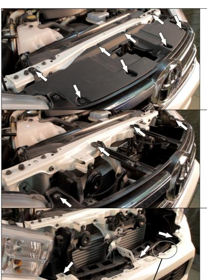
1. Open the bonnet and remove all scrivets holding the grille in place.
