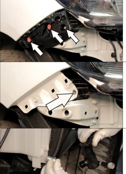
12. Remove M6 bolts and scrivets. Remove plastic side fittings.
