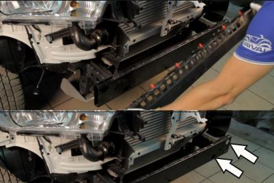
9. Forcefully pull the plastic crush absorber towards you and remove it.
