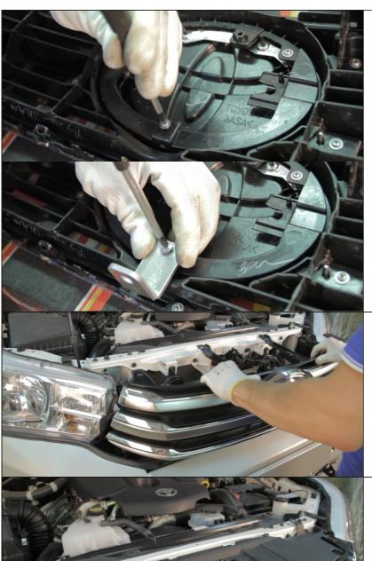
39. Remove lower screw out of radiator grill. Mount supplied bracket (17) using 4.2x16 screw (33) from fitting kit.
