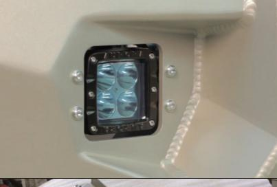
34. Install brackets with LED lights. Fix them with M6x16 round-head screws (26) and M6x12 washers.
